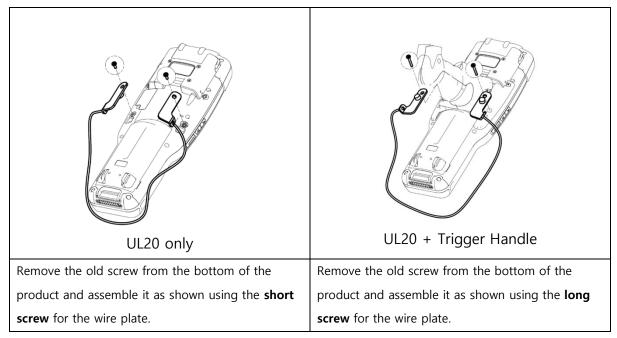
Note! As the direction of assembling the wire plate is different, please refer to the picture.
